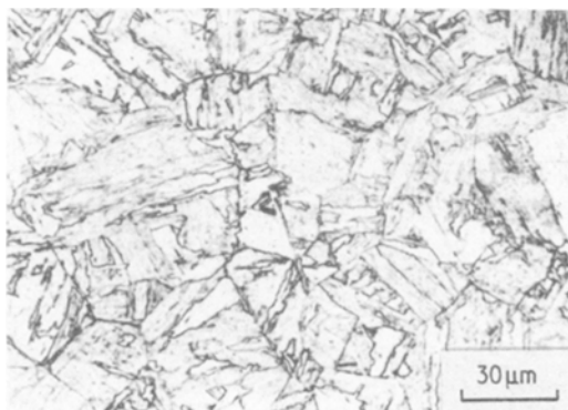
Figure 3 Optical micrograph of the tempered martensitic structure.
